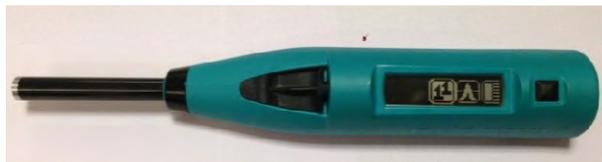
**Fig. 1. Silver Schmidt rebounds hammer Impact energy 2.207 Nm Type N (10 - 100 Mpa)**
