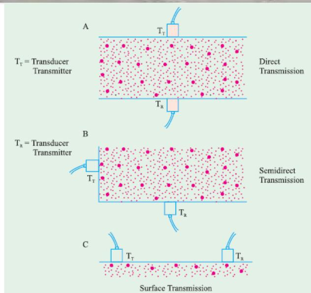
**Fig. 5: Ultrasonic pulse velocity tester      Fig. 6. Type of measurement (A) Direct, (B) Semi-Direct, (C) Indirect**
