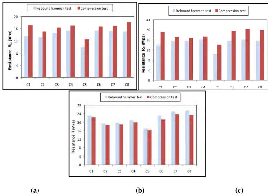
Fig. 4: Effect of destructive and non-destructive tests on the resistance of concrete at the ages of: (a) 7 days, (b) 14 days, (c) 28 days
