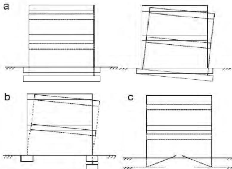
Fig. 2. Different structure settlement scenarios upon soil liquefaction (after [26]). (a) Uniform vertical settlement (left) and rigid-body rotation (right) of a structure. (b) Differential settlement. (c) Possible foundation failure.
