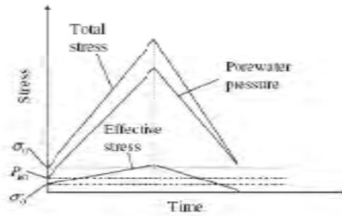
Fig. 1. Schematic of variation of total stress, porewater pressure, and effective stress during a dynamic response leading to liquefaction.
